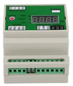
AG-LLM1 Location water leak controller can detect 1500m sensing cable. It'll alarm by flash and sound once there's water leaks on the cable, and the leakage point will display on the LCD screen and the relays will be on automatically.
